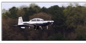
The T-6A Texan II is a single engine, two-seat primary trainer designed to train students in basic flying skills common to USAF pilots. Produced by Raytheon Aircraft, the T-6A Texan II is a military trainer version of Raytheon's Beech/Pilatus Mk II. Columbus AFB received its first T-6 in October 2006 and now has 100 Texans in inventory.
