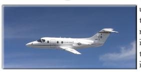
The T-1A Jayhawk is a medium range, twin-engine jet trainer used in the advanced phase of SUPT for students selected to fly airlift or tanker aircraft. The swept-wing T-1A is a military version of the Beech 400A. The T-1A differs from its commercial counterpart with structural enhancements that provide for a large number of landings per flight hour, increased bird strike resistance and an additional fuselage fuel tank. Columbus AFB has 47 Jayhawks.
